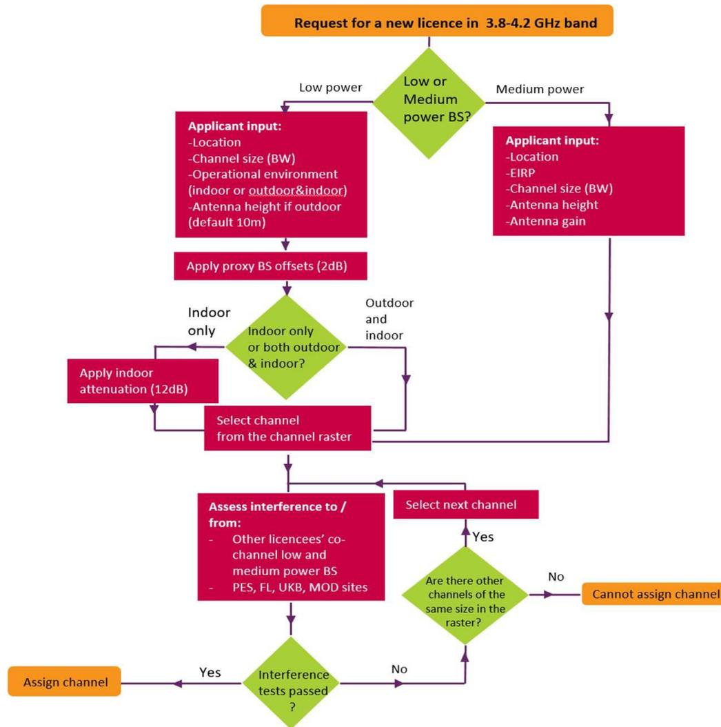
**Figure 23: Ofcom’s proposed coordination approach for low- and medium-power shared access to 3.8-4.2 GHz band.**<sup>124</sup>
