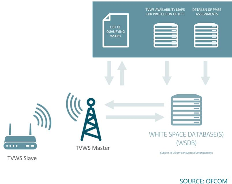
**Figure 11: OFCOM's architecture for Television Whitespace Database (TVDB).**
