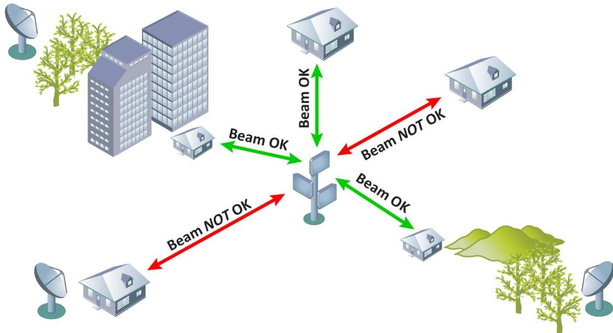
**Figure 22: Automated frequency coordination of directional PtP fixed wireless with FSS earth stations. Unlike mobile use, fixed PtMP is inherently directional and can be sectorized to coexist with FSS.**
