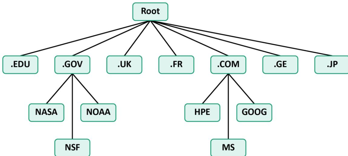
*Figure 3: The Internet's Domain Name Service (DNS) is a distributed database process that connects domain names to IP addresses to facilitate the routing of Internet traffic.<sup>13</sup>*
