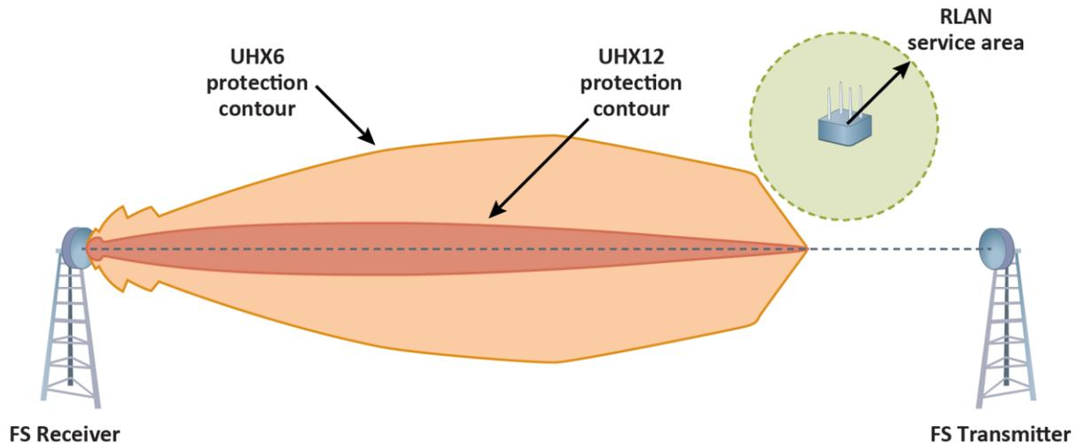
**Figure 20: The AFC system enforces 3D Protection contours to avoid RLAN interference to Fixed Service receivers.**<sup>110</sup>
