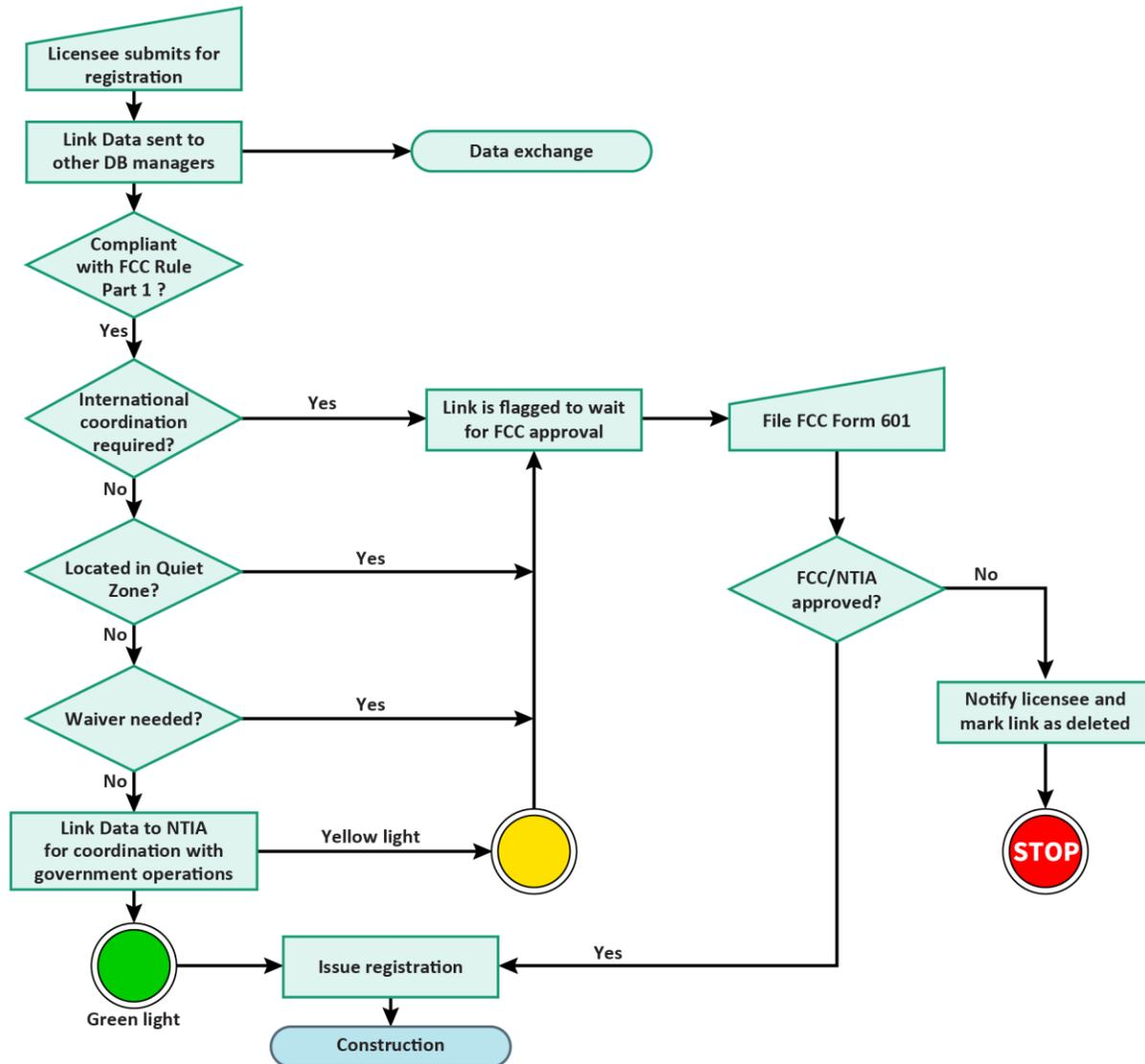
**Figure 7: The 70/80/90 GHz link registration and database coordination process interconnects with a U.S. government database to ensure no conflicts with military or other agency use of the band.<sup>41</sup>**
