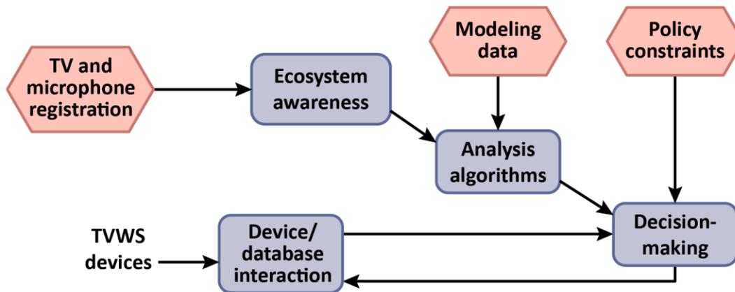
**Fig 10: Simplified admission control system architecture for Television Whitespace Database (TVDB).**
